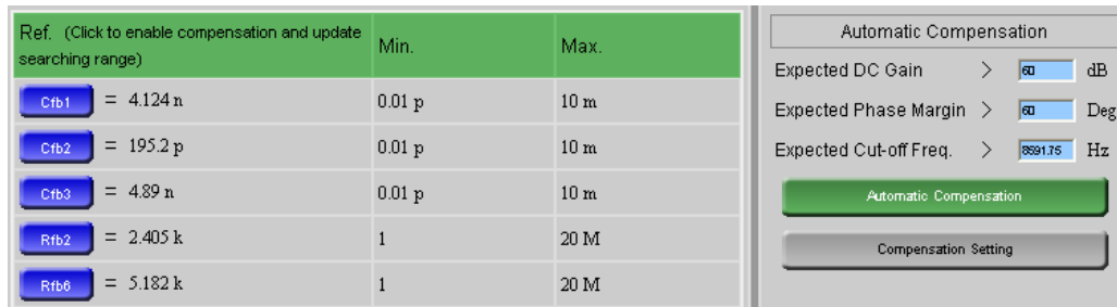
Figure 2.7: Compensation table of proposed buck DC-DC converter.
